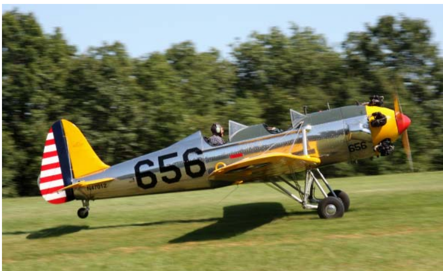
A restored PT-22 shows the classic lines and unique landing gear of the Ryan built trainer. (Charles E. Stewart photo from the AAHS photo archives, AAHS-P001531)
