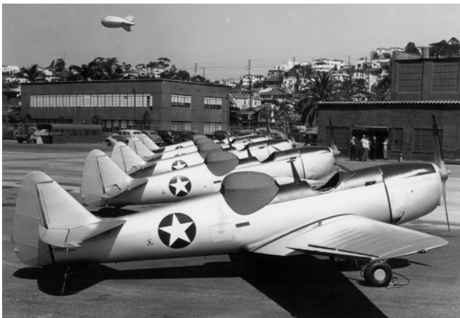
All five Ryan YPT-25s at the factory on Lindbergh Field, San Diego, Calif., with instrument training hoods in place. The design was a plywood version of the PT-22 powered by a 180-hp Lycoming engine. (Ryan photo from the Ed Stoltz collection in the AAHS photo archives, AAHS-P000208)
